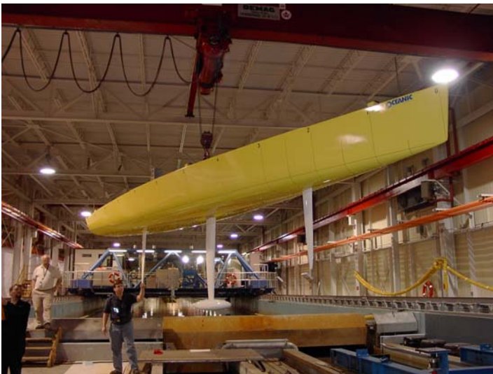
Figure 10 – 1:4 Scale Model of a Modern Racing Yacht Prior to Installation at IOT (Photo Courtesy of Reichel/Pugh Yacht Design)
