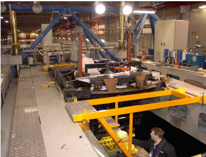
Figure 6 – Towing Carriage at IOT Showing Installed Yacht Dynamometer 2004
