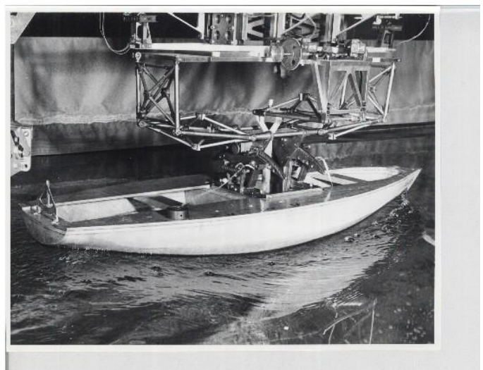
Figure 5 – Small-Model Setup at Davidson Laboratory Tank 1 circa 1970 (Photo Courtesy of Davidson Laboratory)
