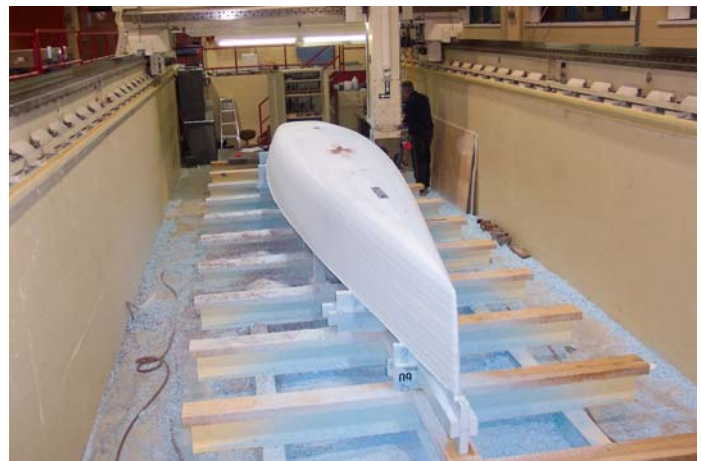
Figure 8 – Large Maxi Racing Yacht Model Setup in Mill (Photo Courtesy of NRC Institute for Ocean Technology)
