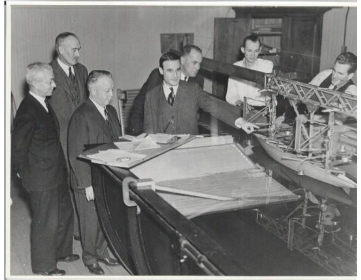
Figure 3 – Ken Davidson Demonstrating the Stevens Institute Tank 1 Yacht Dynamometer (Photo Courtesy of Davidson Laboratory)
