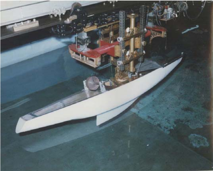
Figure 9 – 1:8 Scale 12 Meter Model (Photo Courtesy of Davidson Laboratory)
